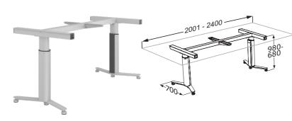
Electric lift for freestanding worktop. For worktops from 2001 - 2400 mm. Height adjustable 300 mm. Including 2 telescopic legs, brackets, longitudinal and cross bracesand switch.
