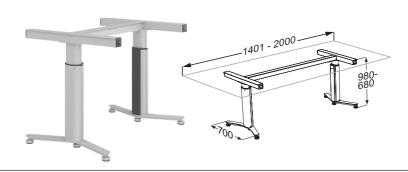
Electric lift for freestanding worktop. For worktops from 1400 - 2000 mm. Height adjustable 300 mm. Including 2 telescopic legs, longitudinal and cross braces and switch.
