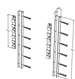
Brackets for wall cupboards, height adjustable by 460 mm. Incl. 2 wall fittings and 2 brackets.
