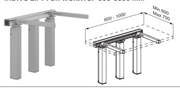
INDIVO lift for worktop, with three motors and control box. Incl. cross brace and two brackets. Height adjustable up to 300 mm with switch or wired remote control. For worktop length 600-1000 mm.
