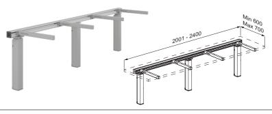
INDIVO lift for worktop, with three motors and control box. Incl. cross brace and four brackets. Height adjustable up to 300 mm with switch or wired
