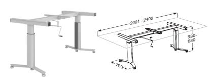
Manual lift for freestanding worktop. For worktops from 2001 - 2400 mm. Height adjustable 300 mm. Including 2 telescopic legs, brackets, longitudinal and cross bracesand crank handle.
