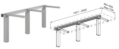
INDIVO lift for worktop, with three motors and control box. Incl. cross brace and three brackets. Height adjustable up to 300 mm with switch or wired
