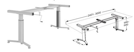
Manual lift for freestanding worktop. For worktops from 2401 - 3000 mm. Height adjustable 300 mm. Including 2 telescopic legs, brackets, longitudinal and cross bracesand crank handle.
