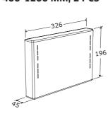
Extension fittings, 400-1200 mm, 2 pcs. For installing cupboards higher than 704 mm. For INDIVO lift for wall cupboards.
